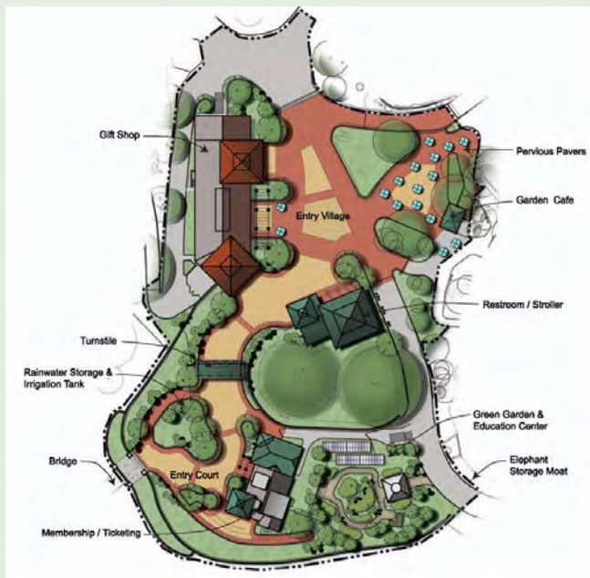
Cincinnati Zoo New Main Entry with MSD-Funded Storm Water Control
