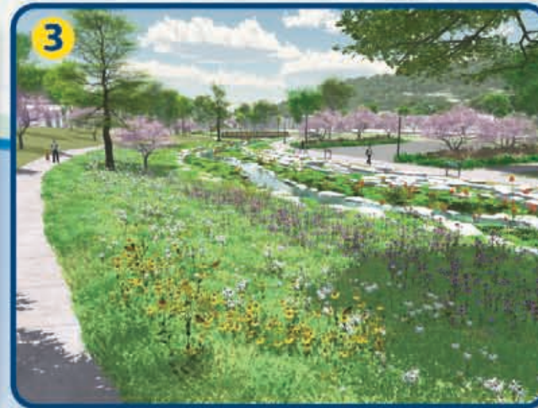
(Looking Northwest) This image depicts the character of the proposed urban waterway near the Civic Recreation Hub. Native vegetation is included to help reduce maintenance needs and to provide water quality benefits during high flow events. The pedestrian bridge in the background is above the modeled 100-year floodplain elevation; so during large volume rain events, water elevations would be contained within the heavily-planted areas.
